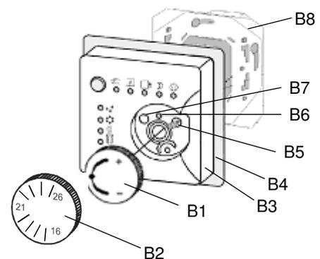
figure 2: Mounting controller
