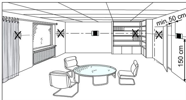
figure 3: Installation references for sensors and temperature controller.
