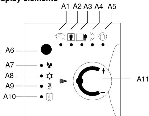
figure 1: Location of the operating and display elements
