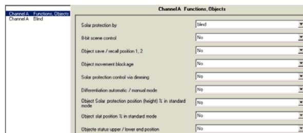
This parameter window provides selection of the basic function (solar protection via Venetian blind or roller shutter/awning) and further functions of this actuator output. This includes
