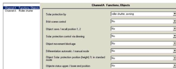
This parameter window provides selection of the basic function (solar protection via Venetian blind or roller shutter/awning) and further functions of this actuator output. This includes
