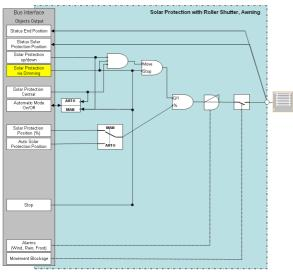
Function roller shutter/awning, sloar protection via dimming
