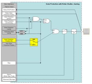
Function roller shutter/awning, solar protection position
