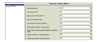
This parameter window provides selection of the basic function (solar protection via Venetian blind or roller shutter/awning) and further functions of this actuator output. This includes
