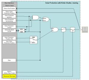
Function roller shutter/awning, movement blockage
