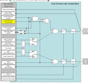
Function blind, solar protection via dimming
