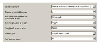
The function "1-button multi-touch control (multiple output control)" enables targeted switching of up to 2 resp. 3 load groups using just one push button. The number of push button switching actions immediately following each other determines, which load group is switched:
