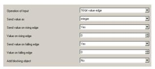
This function is used to send 16-bit integer values (DPT 7.001) ranging from 0...65535 or 16-bit floating point values (DPT 9.000) ranging from -3276.8 to 3276.7 (with one decimal place). The exponent of the 16-bit floating point value is automatically generated. An adjustment can be made as to whether a value telegram is to be sent as a reaction to a rising and / or falling signal edge on the channel input (i.e. when a push button is pressed and / or released).
