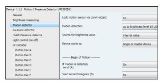
In the following paragraphs the parameters for the functional block "Motion detector" are described. The configuration for the functional block "Presence detector" is performed similar.
