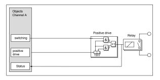
The positive drive object is a 2-bit object. Bit 1 determines, whether positive drive is "active" (= 1) or "passive" (= 0).
