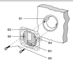
Figure 2: Mounting the bus coupling unit UP 110/11
