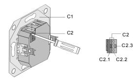
Figure 3: Slipping off/on bus connection blocks
