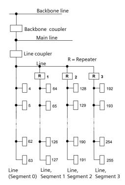
Figure 1. Connection of repeaters to a bus line
