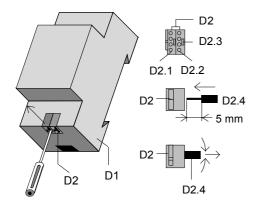
Figure 4: Connecting / disconnecting bus cables
