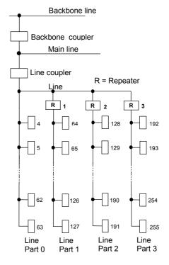
Figure 1. Connection of repeaters to a bus line
