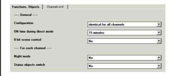
If individual parameterization per channel is desired and parameters for more functions and objects set to "Yes", then an additional parameter will be shown on this parameter page and more parameter pages added (see the following graphic).
