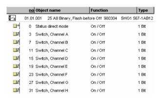
The following 34 communication objects are shown for the 8-fold switching actuator N 567/12 when all additional functions were activated.
