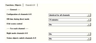
If individual configuration per channel is desired and parameters for more functions and objects set to "Yes", then an additional parameter will be shown on this parameter window and more parameter windows added (see the following graphic).
