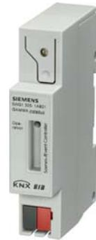
The N 305 scenes-/event controller is a device for DIN-rail mounting with N-system dimensions 1SU wide. The controller's application program includes scenes control and event program functions, either of which can be selected while setting the parameters.
