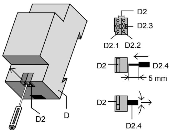
Figure D: Plugging in/removing the bus terminal
