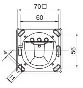
Dimensions surface Frame for PresenceLight 360x-KNX, PresenceLight 180x-KNX
