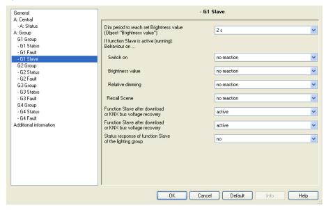
With operating function *Slave*, the lighting follows the Brightness value provided by the master via the communication object *Brightness value of slave*. The reaction to switch, dim or brightness value telegrams can be parameterised individually.
