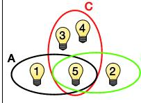
Group A dimming thresholds: 1...100 % Group B dimming thresholds: 20...80 % Group C dimming thresholds: 30...70 %
