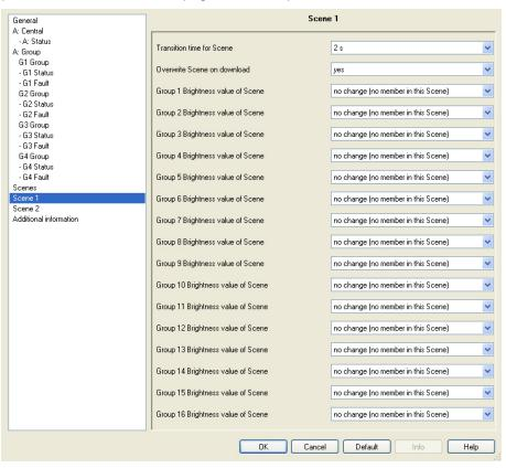
A scene value must be assigned in order to set a scene value for the lighting group. The scene value complies with the brightness value, which the lighting group assumes when the scene is recalled.
