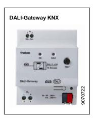
The group-oriented DALI-Gateway KNX is a modular installation device. Up to 64 DALI devices that can be controlled in 16 lighting groups may be connected to a DALI output.
