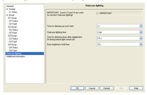
The Gateway features a function *Staircase lighting* which can be triggered and stopped via individual switch telegrams of the individual lighting groups.
