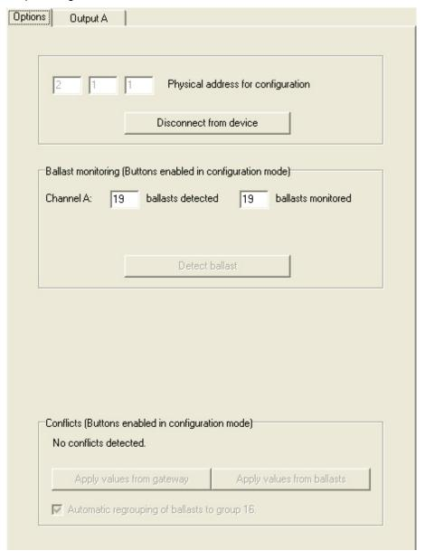
The field *Device monitoring (fields enabled in configuration mode)* indicates how many DALI devices have been detected by the Gateway and the number being monitored. If the number detected does not correspond with the number of monitored DALI devices, the Gateway cannot undertake correct ballast monitoring.
