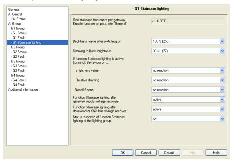
The Gateway features a function *Staircase lighting* which can be triggered and stopped via individual switch telegrams of the individual lighting groups. For each Gateway a Staircase lighting sequence can be programmed which can be adjusted in the parameter window *Staircase lighting*, page 97.
