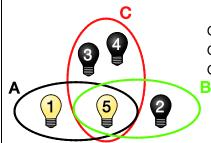
Group A dimming thresholds: 1...100 % Group B dimming thresholds: 20...80 % Group C dimming thresholds: 30...70 %
