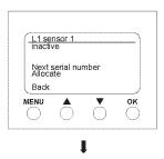
Allocate new serial number to inactive sensor
