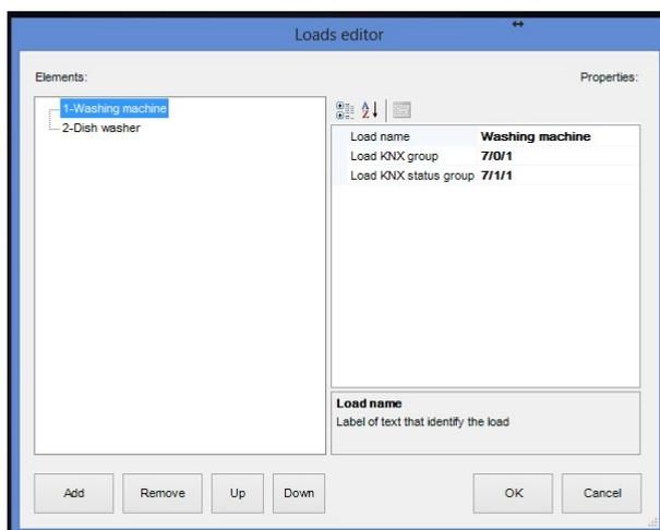
Loads editor window: load number 1 is the first load to be disconnected
