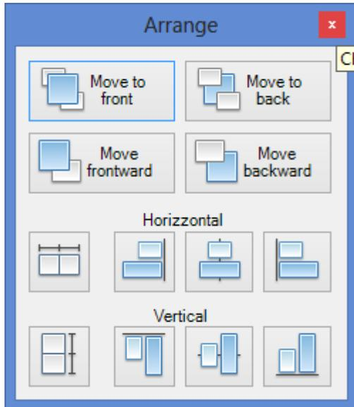
As the view of the objects on the webpage and on the vertical view on the iPad is determined by their position within the structure of the project (Interface window) it may be necessary to move them up and down within the structure, f.e. to to group all the commands of a certain room. This can be done using the “move frontward” and “move backward” commands, which you find clicking the “Arrange” button. With the same method you can change the position of the pages within the function.
