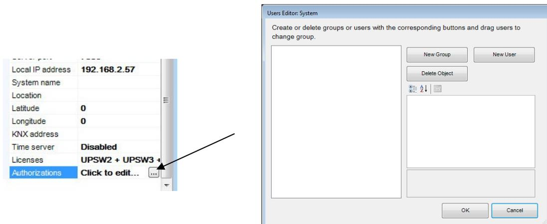
Create a new group by clicking the "New Group" button. In the users tree you will see a new entry with a standard name. To change the name select the new entry and in the properties grid type the new name in the proper field. The updated name will immediately appear in the users tree.
