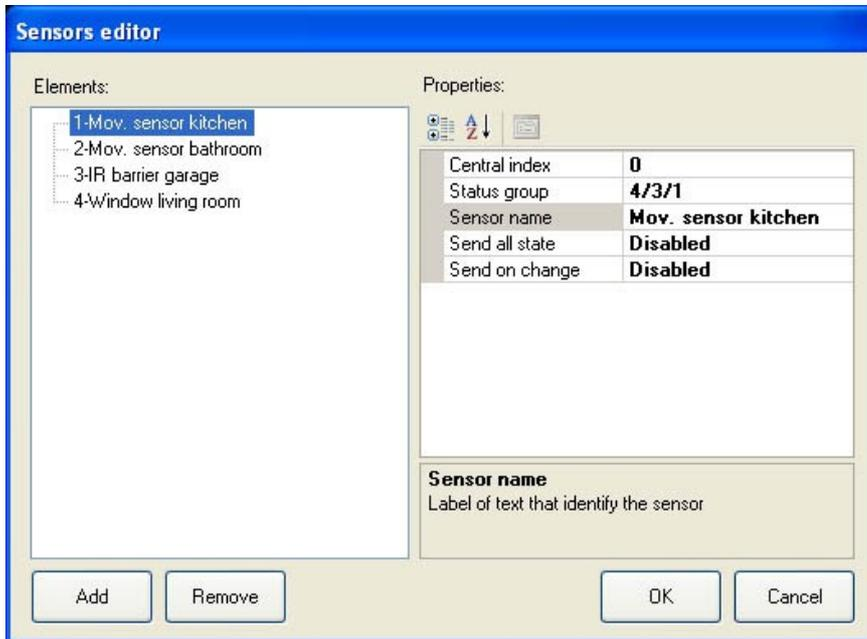
Index number: insert the number of the sensor you programmed in your security system. ATTENTION: Numbering in configurator always starts with "0", if the first sensor in your security system has number 1 this corresponds to number 0 in configurator.
