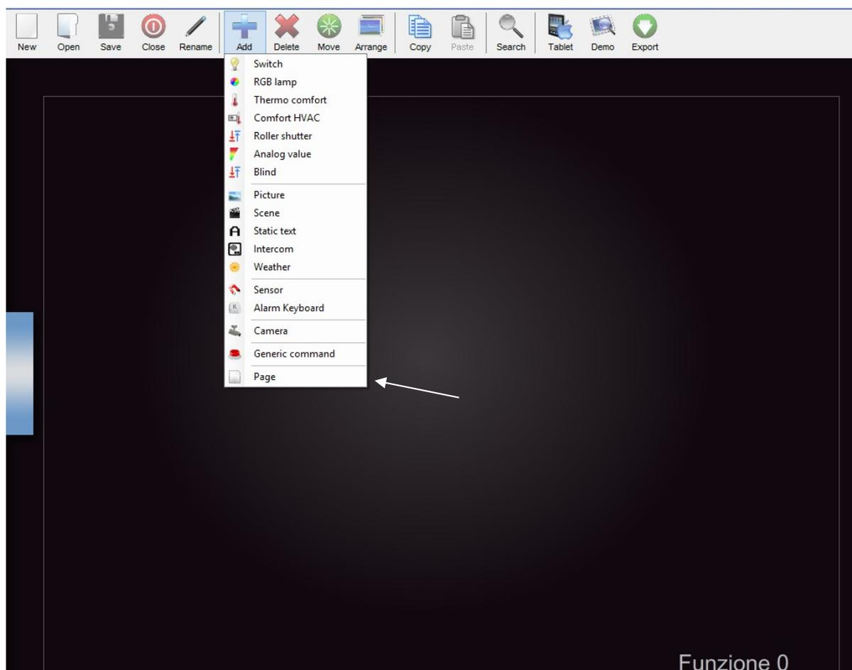
Each page created, automatically shows up on the top bar starting from the left, the only limitation on the number of pages you can create is the number of characters that can be shown on the top bar. The longer the names of the pages, the less pages you can create.
