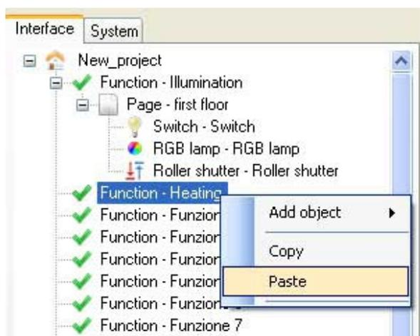
In this example we have copied the page “first floor” contained in the function “Illumination” and are going to paste it into the function “Heating”
