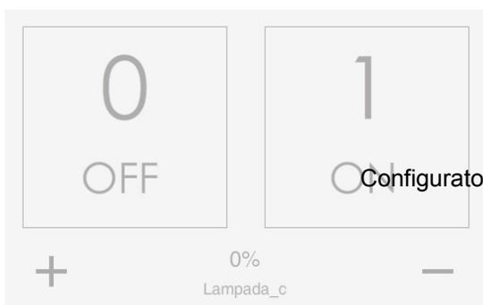
If you select “Dimmer” as type of command the KNX groups “value” and “value feedback” are added. Select the corresponding group addresses (1 byte) of the imported ETS project. On the client interface the dimming popup is automatically activated.
