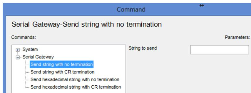
**Send string with no termination:** Sends the string in alphanumeric format without “carriage return” at the end of the command.
