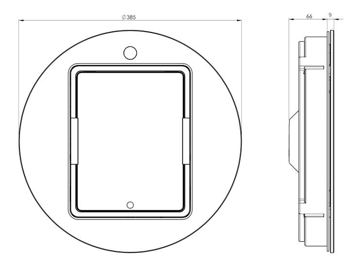
Cutting measurements for solid, concrete and hollow walls, (for the wall case), in mm
