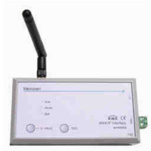
Photo: KNX IP Interface 740 *wireless*
