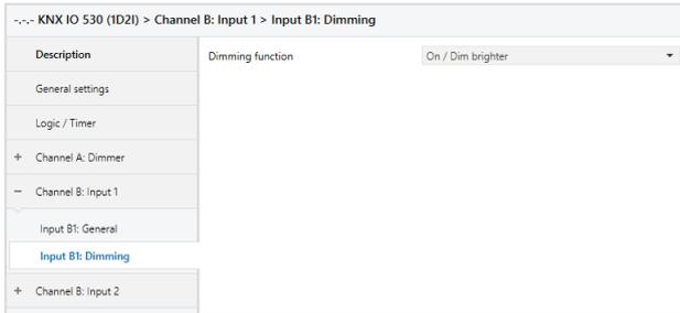
On selection of function Dimming following objects are visible:
