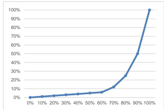
The output values are fixed for the "Linear" and "Logarithmic" dimming curves, and can be freely configured for the "User-defined" curves.
