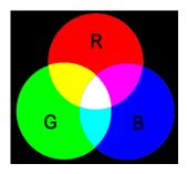
Figure 3. Combination of the Red, Green and Blue colour components
