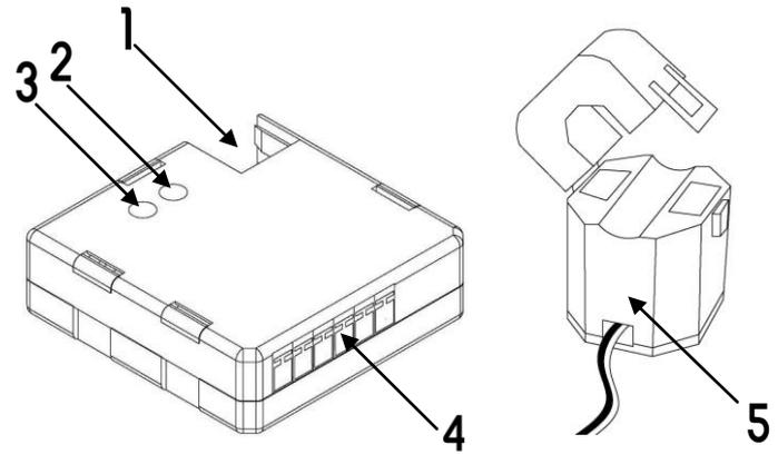
**Programming button:** push button to set the programming mode. If this button is held while plugging the device into the KNX bus, it goes into secure mode.
