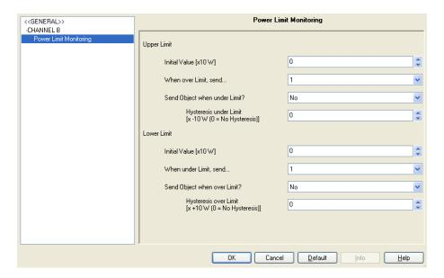
Figure 11 Power Limit Monitoring.
