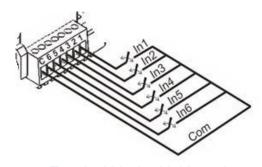
Figure 5. Terminal block with binary inputs
