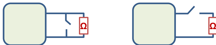
Figure 4. Left: normally open Sensor (parallel resistor). Right: Normally Closed Sensor (serial resistor).
