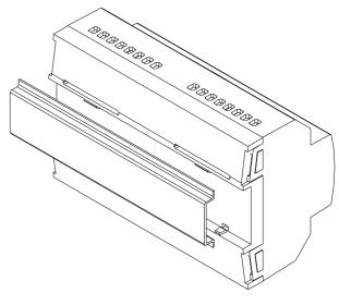
Figure 3. Mounting MAXinBOX SHUTTER 8CH on a DIN rail
