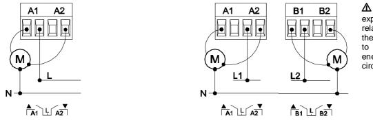
▲ In order to ensure the expected status of the relays, please check that the device is connected to the KNX bus before energizing the power circuit.
