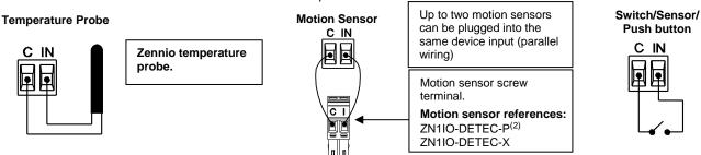
(2) The micro switch number 2 in the ZN1IO-DETEC-P sensor must be in Type B position to work properly.
