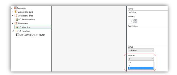
Figure 17 Zennio KNX-IP Router PLess as a Line Coupler.
