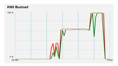
Figure 10 Web interface (KNX bus load)
