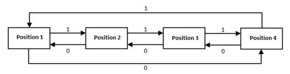
Figure 15. Cyclical flap step control (4 positions and no swing function)
