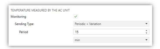
Figure 6. AC Gateway. Configuration. Temperature measured by the AC unit.
