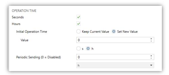
Figure 10. AC Gateway. Configuration. Operating time.
