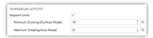
Figure 7. AC Gateway. Configuration. Temperature setpoint.
