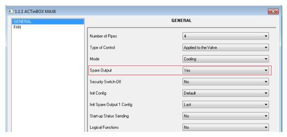
Figure 3.12. Spare output in a 4-pipe system
