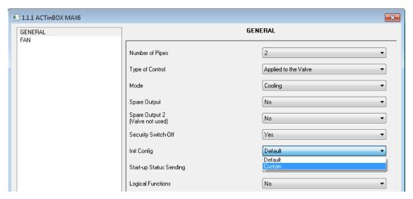
Figure 3.15. Fan Coil start-up configuration
