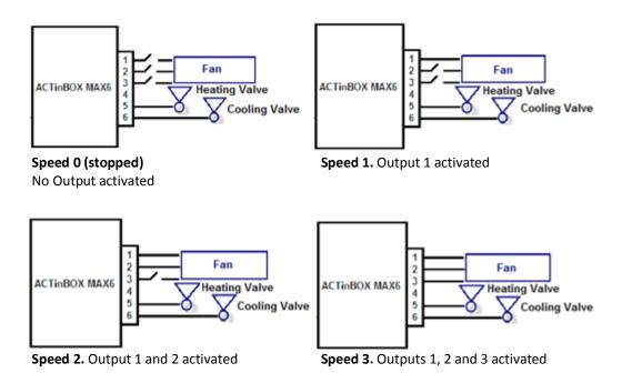
Figure 3.6. Ventilation speed control by accumulation
