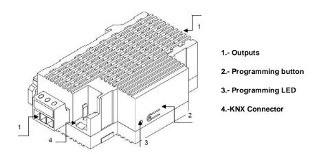
Figure 1.2. ACTinBOX MAX6. Elements scheme
