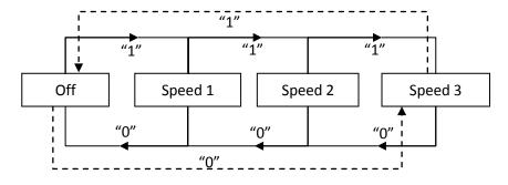
Figure 2.2. Cyclical manual step control
