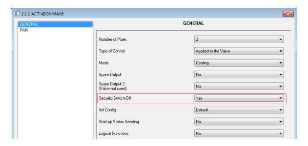
Figure 3.14. Security switch-off
