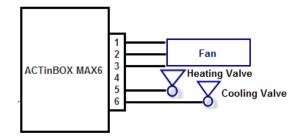
Figure 1.3. ACTinBOX MAX6 to 4-pipe Fan Coil connection
