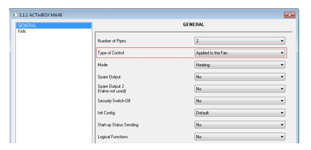
Figure 3.3 Type of control selection: applied to the fan
