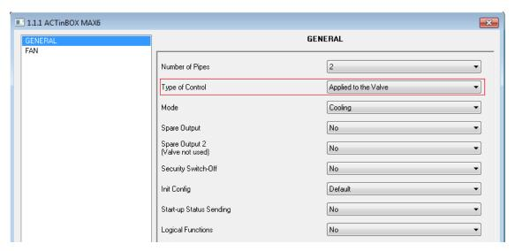
Figure 3.7. Type of control selection: applied to the valve
