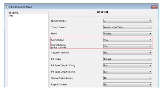
Figure 3.13. Spare outputs 1 and 2 in a 2-pipe system
