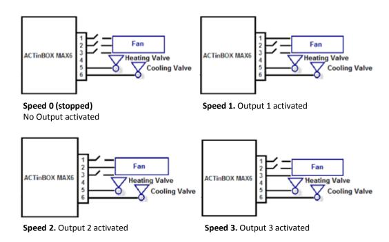
Figure 3.5. Ventilation speed control by switching
