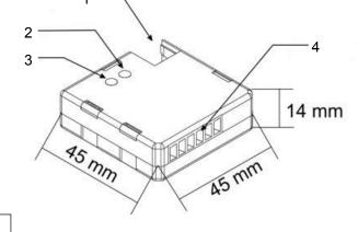
1. KNX bus 2. LED 3. Programming button 4. Socket
