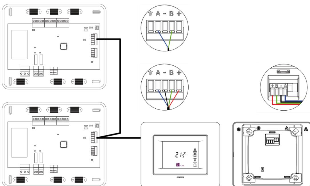
Wall-embedded Supermaster have a 5-pin terminal on their back part. Attach the wires with the terminal screws following the color code.
