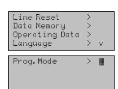
Move the cursor (flashing rectangle at right edge) to the "Prog. Mode" menu with the keys  $\nabla$  and  $\triangle$  and confirm with the key  $\triangleright$ .
